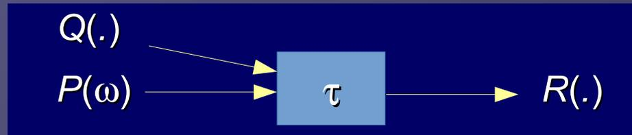
so that the functional behavior of the device is actually twofold, a transduction  $\tau$  preceded by a filtering  $\varphi$ :
