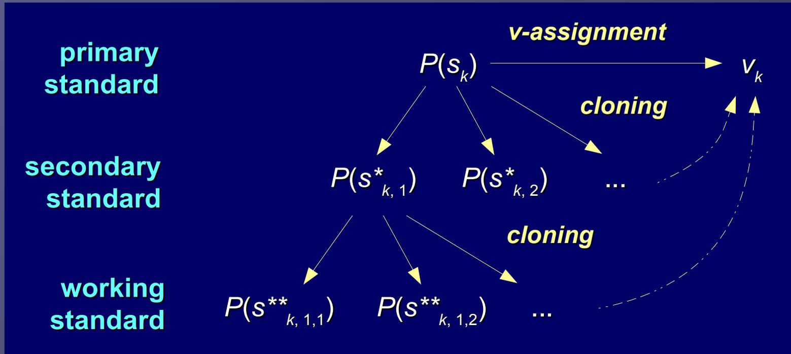
**Each cloning process is a standard calibration**
