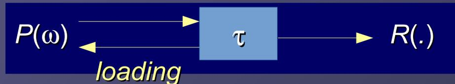
so that what is measured is not the unaffected state of  $\omega$  but a modified version of it (despite the operative similarity, this has nothing to do with the situations “of signal conditioning” in which  $\omega$  has to be modified on purpose before measurement so to make the measurand properly accessible to  $\tau$ )
