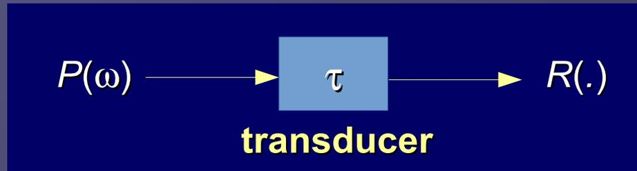
It is assumed that such output property  $R(.)$  (traditionally called “**instrument reading**” or “**indication**”) conveys sufficient information on  $P(\omega)$
